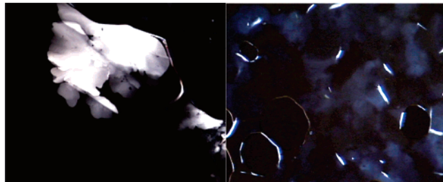
Figure 2. PLM images (left: ILC 8a , right: ILC 8b ) were obtained as LC phases and appeared upon cooling from the isotropic melt; magnification = 100 \times .
